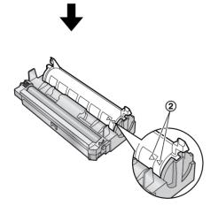
6 Remove the used cartridge (①) from the drum unit (②).
